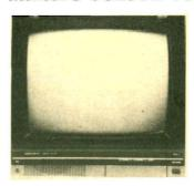
The Mikado colour television receiver (Model CTV 5101) employs the newly designed single chip LSI circuit which contains a microprocessor, PCM remote control and a non volatile memory for voltage synthesizer tuning. The tuning system precisely tunes to VHF channels 2 to 4 and 5 to 12 and UHF channels 21 to 69. It can also memorize upto 12 stations on either the VHF or UHF wavebands.
